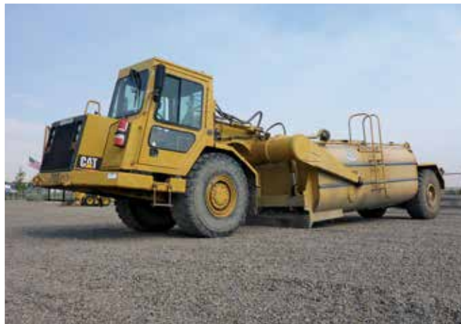
Caterpillar 613C Series II 5000 Gallon Drop Tank
